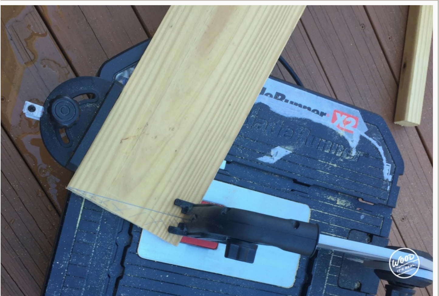
The most important angle cut here will be the little one at the top, which will allow an angled armrest later on in the build.
