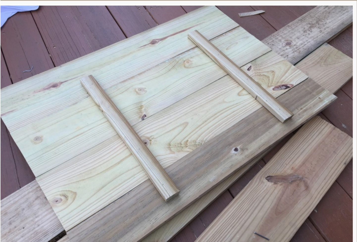
Measure 3 or so inches in from the outside of the lid frame boards to attach the cleats.
