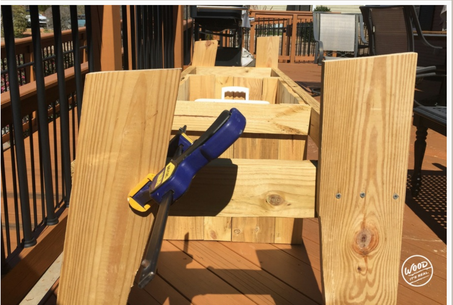
To make sure you have the back legs in the right spot, you'll test the angle of the arms using a flat board on the top to keep the height and angles correct.
